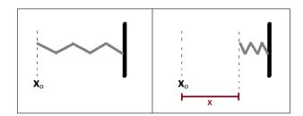
27. A horizontal spring is initially unstretched with its right edge connected to a vertical post, and its left edge resting at position Xo, as shown in the image above left. A moment later, the spring is compressed, and its left edge is now located a distance X measured to the right of Xo, as shown in the image above right. Which graph below correctly analyzes the potential energy stored in the spring U as a function of the position of the springs left edge?
